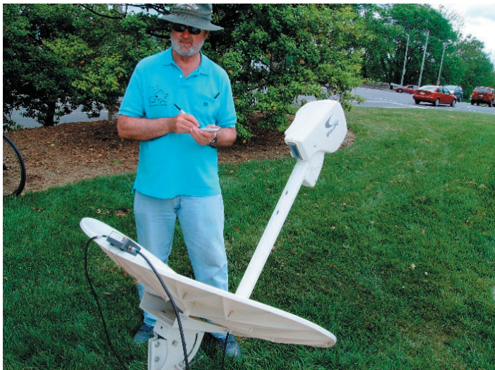
Dave Thomas calibrates the field of reception of his radio telescope, after people walked in front. This calibration involved timing the drift of the Sun across the receptor, while measuring signal strength.
